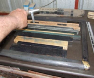
Locking up a cutting forme
