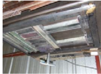
Locked up job on a chase ready for printing
